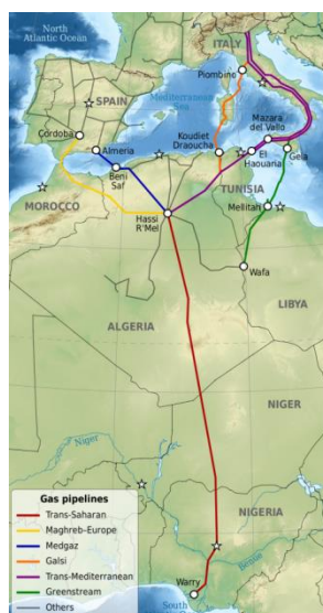
Figure 5: Gas pipelines in North & Central Africa 30
